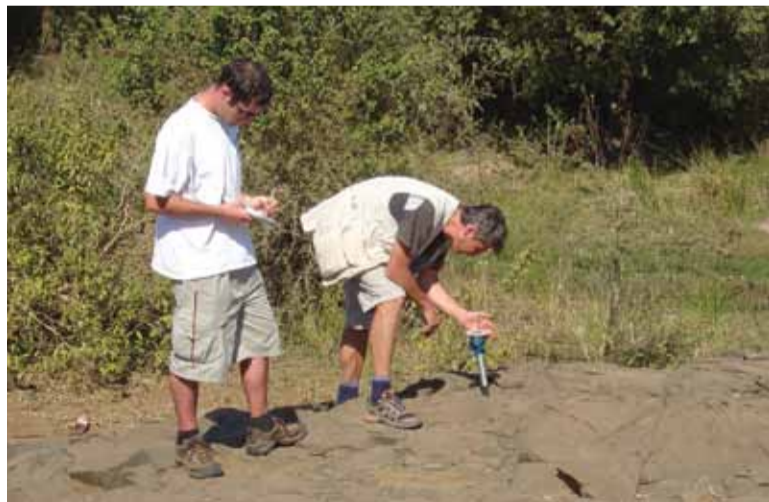
(from left) Mr Warwick Hastie and his French co-supervisor, Dr Charly Aubourg, in Swaziland measuring the orientation of a core of rock that has just been drilled prior to its collection.
